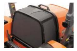
**RADIATOR SCREEN** Kubota has now integrated the radiator screen into the bonnet for better sealing performance and less likelihood of grass clippings finding their way inside the screen.
