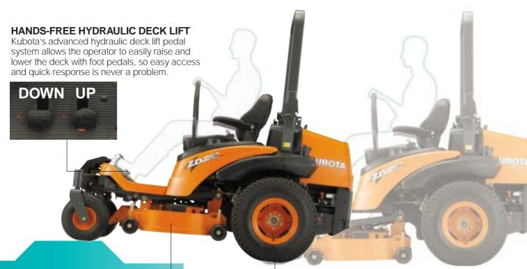
Now you can elevate the mower deck and literally roll right over obstacles, thanks to the ZD-300 mower hydraulic deck lift.
