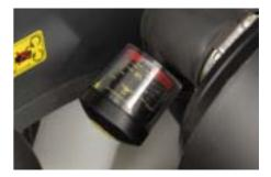
**AIR CLEANER INDICATOR** The ZD-300 features an air cleaner indicator that indicates when it's time to change or clean the filter, and help maintain maximum airflow capacity.
